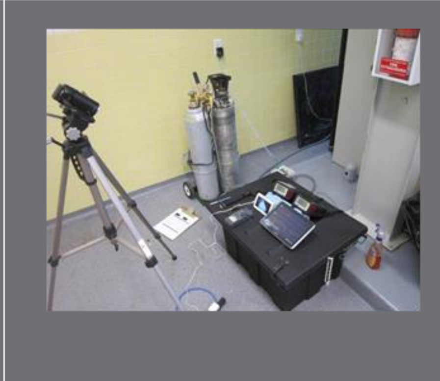
EEG/ECG Set up for Gas/Foam euthanasia devices. (Note gas level recording meters and closed circuit video camera for observations)
